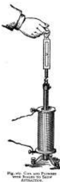
Fig. 267 COIL AND PLUNGER WITH SCALES TO SHOW ATTRACTION.
