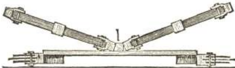
Fig. 228. MAGNETIZATION BY DOUBLE TOUCH.
