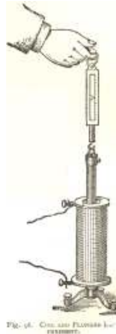
Fig. 96. COIL AND PLUNGER EXPERIMENT.
