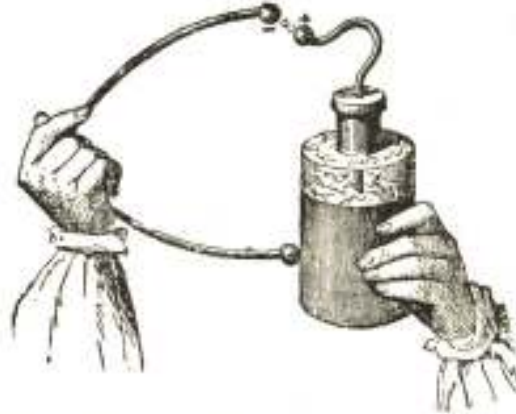
Fig. 213. LEYDEN JAR WITH DISCHARGER.
