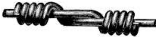
Fig. 203. AMERICAN TWIST JOINT.
