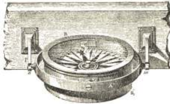
Fig. 191. COMPASS SUSPENDED IN GIMBALS.
